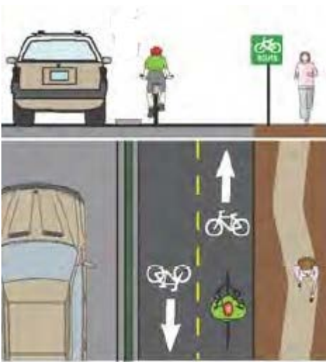
Two-way Bike Path and sidewalk – Aerial view
