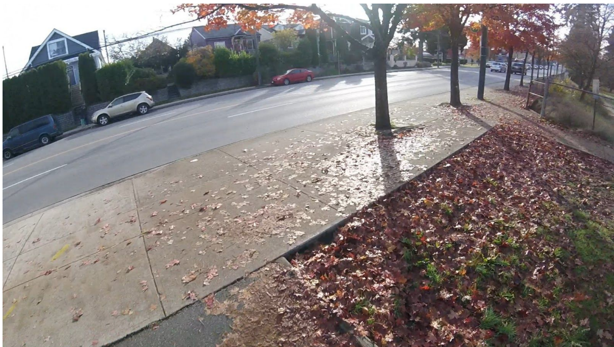
Figure 5 - 37th at Fraser St showing the MUP on the sidewalk. Painted lanes on the MUP along with turn arrow stencils, would improve safety for users of all modes at this corner, as the bike/walk signs are located in the trees along the path, but not at the start of the MUP.
