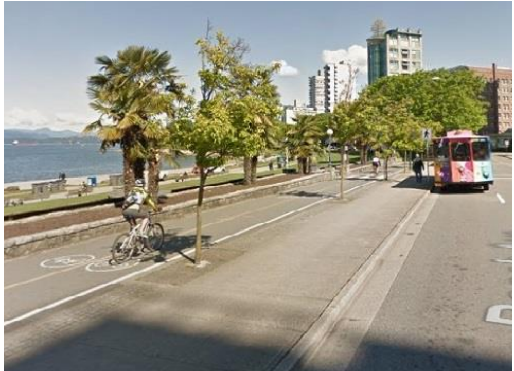
Figure 7: Yellow centre line and stencils to reduce user conflict (Seawall at Beach Avenue, City of Vancouver). The City of North Vancouver uses walk/bike stencils the same way on the Spirit Trail.
