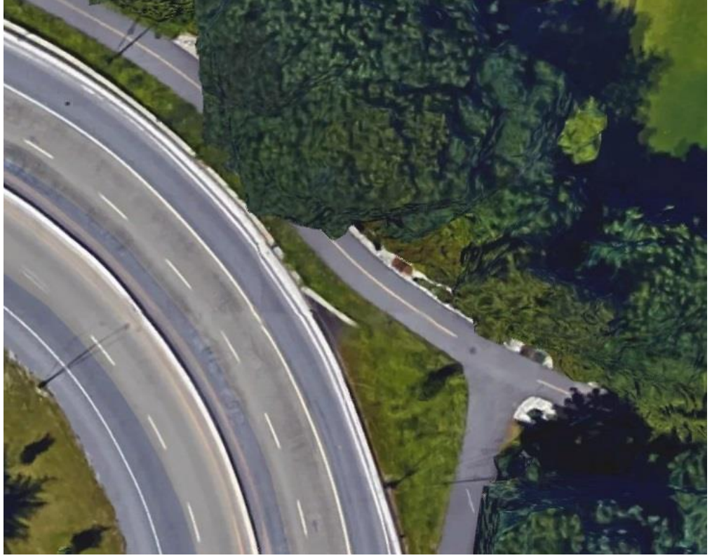
Figure 8: Yellow centre line on two-way multi-use path at Lions Gate Bridge cloverleaf, West Vancouver. Note no centre line is marked on one-way path from Marine Drive (bottom right).
