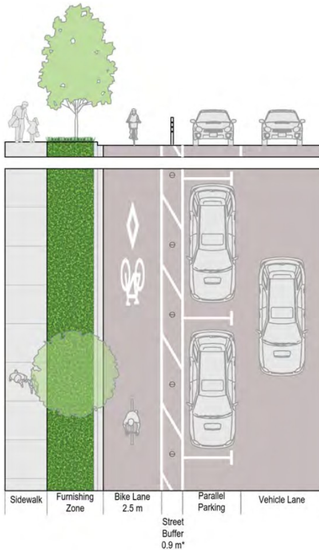
FIGURE D-39 // UNI-DIRECTIONAL PROTECTED BICYCLE LANE CROSS-SECTION - WITH ON-STREET PARKING (DESIRED WIDTH)
