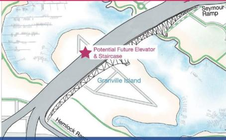
A potential future elevator and staircase to Granville Island and Seawall, served by an intersection and bus stops on the bridge deck
