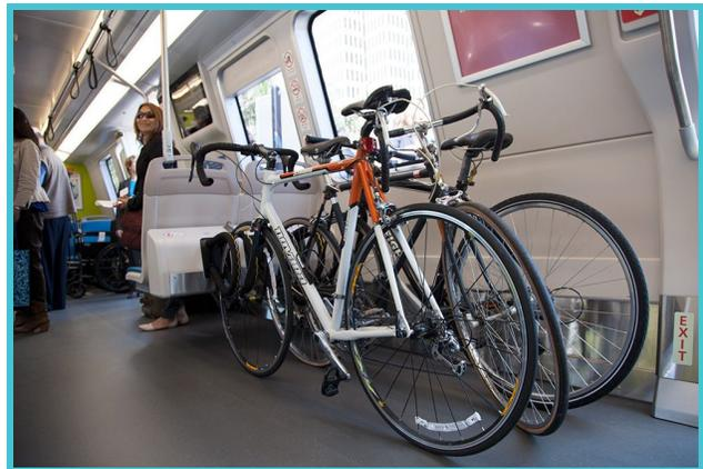
Figure 2 - Bike racks on the BART system stabilize bikes
