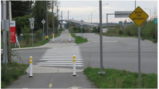
• Apart from the improper placement of bollards we are also concerned about the design of the bollards. All appear to have a base which is raised above the level of the path. If bollards are knocked out or removed this raised lip remains as a virtually invisible hazard.
