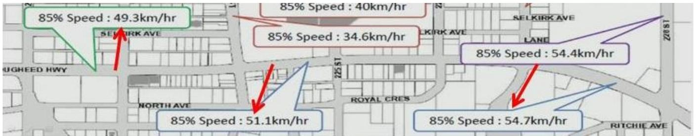
A similar road lay-out is proposed for the section between 224th and 226 Streets, where presently 85% speeds are 51.1 km/h. There is no reason to expect any meaningful reduction in speeds along this section.
