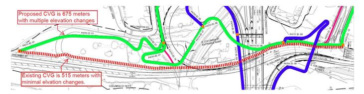
2. A direct overpass connection from the North East end of the new Agnes Greenway to the Eastbound onramp to the bridge. The current design is 20 times longer with multiple elevation changes. Not having this direct connection is a fundamental flaw in the design and needs to be corrected.
