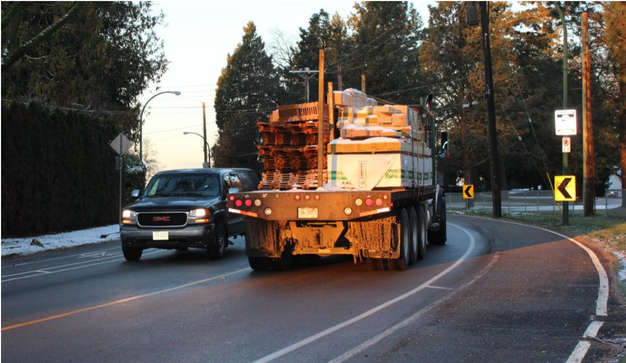
Figure 19: Vehicle Encroaching into the Bicycle Lane While Navigating a Curve in the Road
