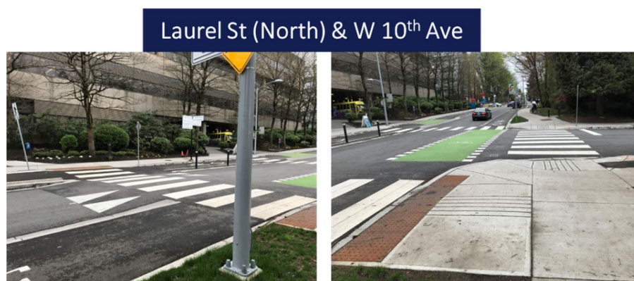
Figure 34. Design complexity pedestrians in front of the Mary Pack Arthritis Centre and the Spinal Cord Centre; varying paving materials can be a challenge, especially for people with disabilities and guide dogs
