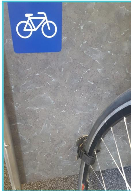
These types of front velcro straps work well on several WCE trains and should be added on all.
