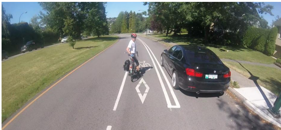
Figure 2 – Bicycle lane positioning to avoid the door zone
