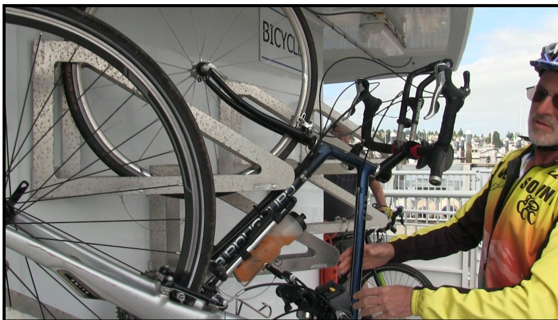
Figure 3. Vertical racks work well if space is limited but are less accessible than horizontal designs. Washington State Ferries
