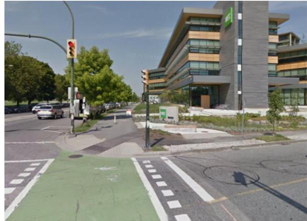
**Figure 3: Central Valley Greenway multi-use path crossing on Great Northern Way at Glen Drive in Vancouver. The shared pedestrian and cyclist crosswalk is marked in green, in addition to elephant's feet.**
