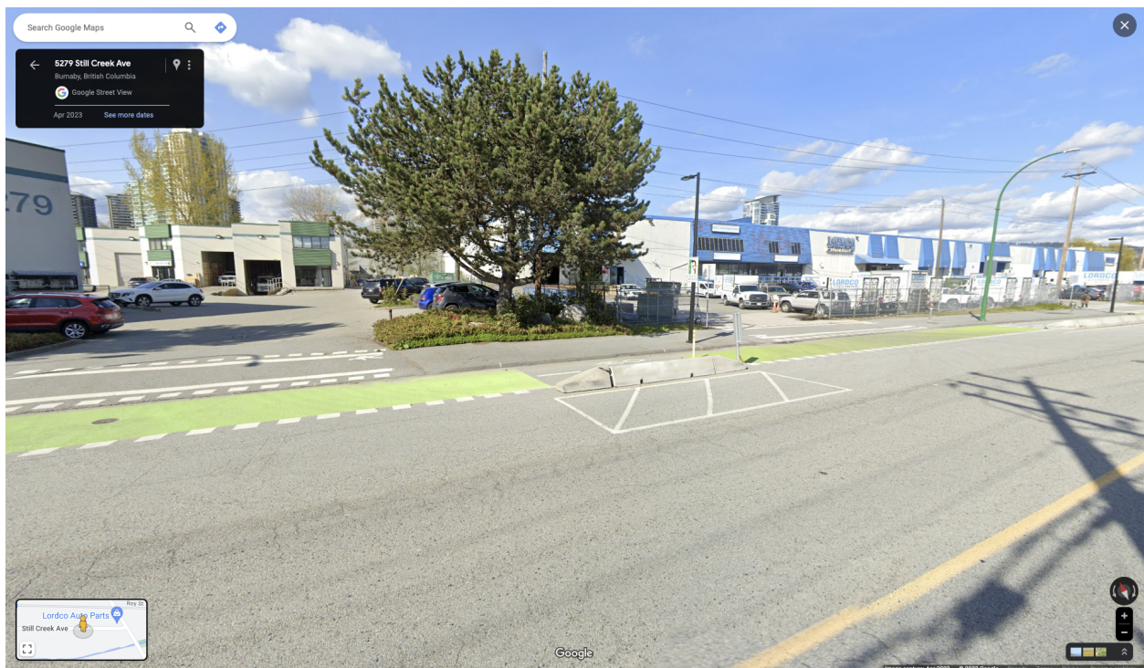
Figure 1: Still Creek Avenue bike facilities are a good example of the green colour treatment.
