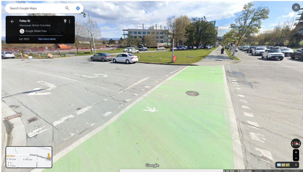
Figure 3: example of the green colour treatment along a MUP from the City of Vancouver along Vancouver's portion of the Central Valley Greenway.
