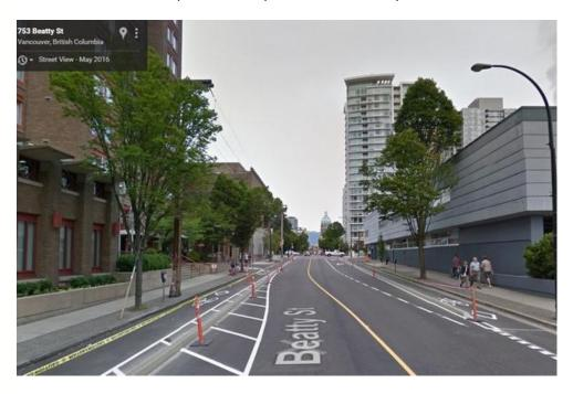
As to the planned parking in segment 3, we would like to point out that the design challenges with a protected multi-use path are similar to those for a protected cycle track. According to the <u>NACTO Urban Bikeway Design Guide</u>, regarding the crossing of minor side streets and driveways: "if the cycle track is parking protected, parking should be prohibited near the intersection to improve visibility. The desirable no-
