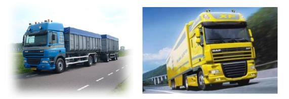
Left a truck with open, right one with closed under-run protection. Closed underrun protection increases safety and can save up to 8% in fuel consumption.
