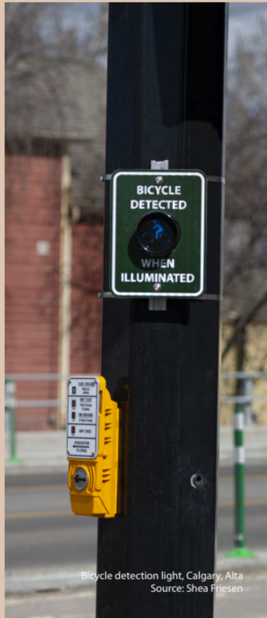
Figure 5. Excerpt from the BC Active Transportation Design Guide 2019. These would eliminate the need for people cycling to dismount to push the call button. This system is used at Eighth St and 8th Ave in New Westminster.
