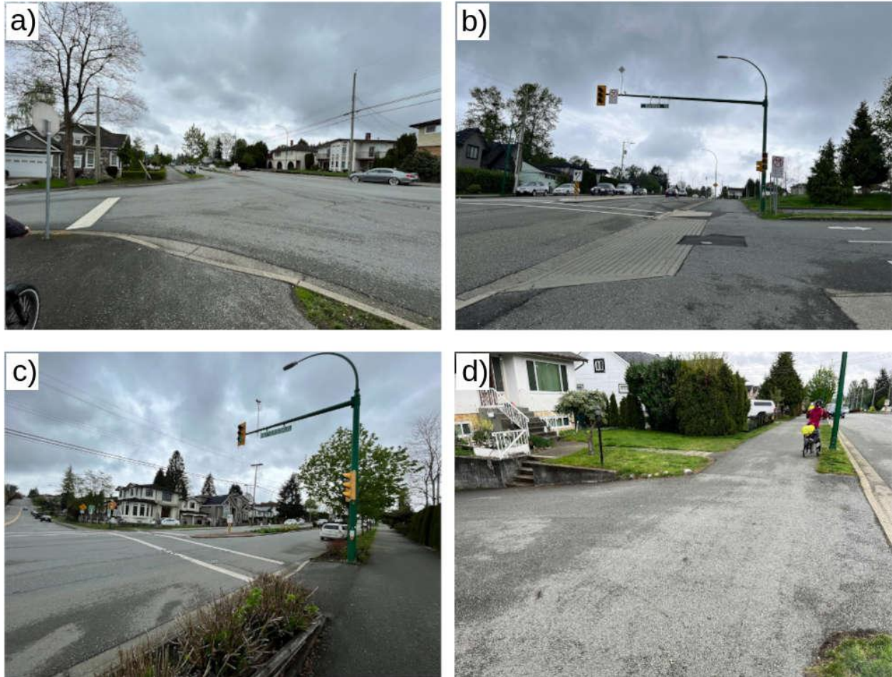
Figure 1. a) Intersection at Moscrop and Inman with no elephant's feet or green conflict paint. b) Crossing at Moscrop Secondary School driveway without green conflict paint. c) Crossing at Patterson and Moscrop connecting two segments of the Sea to River Bikeway does not have elephant's feet or green conflict paint. d) Residential driveway without green conflict paint or other markings.
