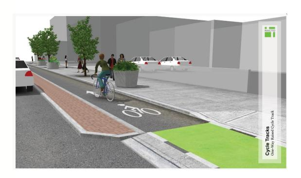
We would like to see a gradually ramped maximum 3" drop from any raised (above grade) path surface down to each driveway entrance surface, with a rounded (filleted) 3" to 4" balance of the drop left for the cars to climb on/off of.
