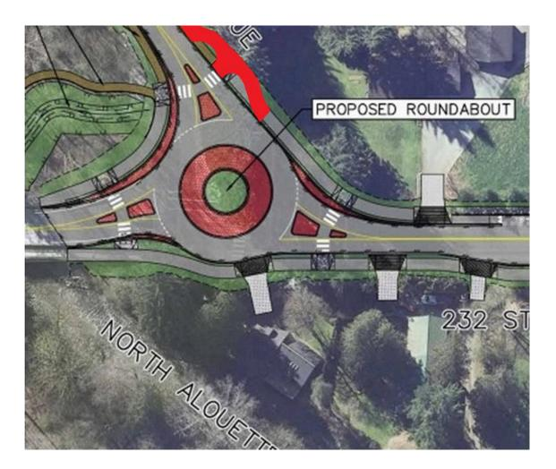
We would also like to see the design of the roundabout changed slightly to add a bit more of a curve on that side to make cars slow down. It would, of course, be preferable to keep any remaining vegetation on this corner if possible, but visibility of cyclists and pedestrians crossing especially at this crossing may be an issue. Slowing down cars will help mitigate this.
